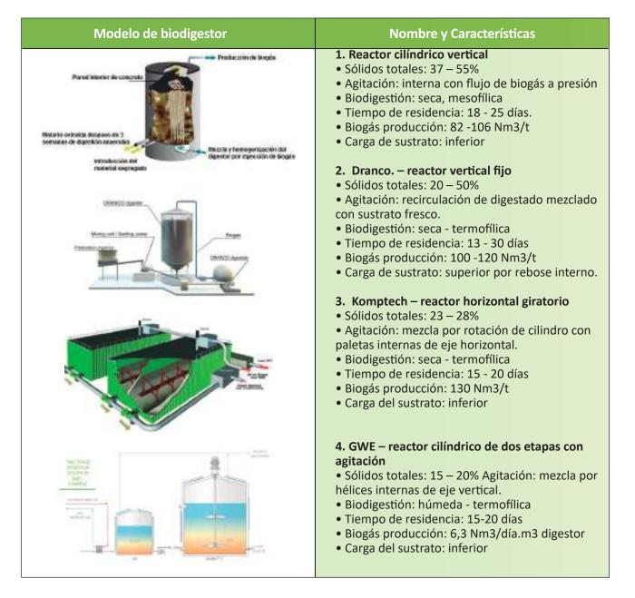
**Tabla 8** Tipos de Biodigestores para Residuos Orgánicos Municipales **Fuente:** biodigestores 1. 2. Y 3: Quevedo/Martins, AnaerobicDigestion of Municipal Solid Waste in Santo André – SP, 2014; biodigestor 4: http://www.globalwe.com/technologies/raptor/ 2019
