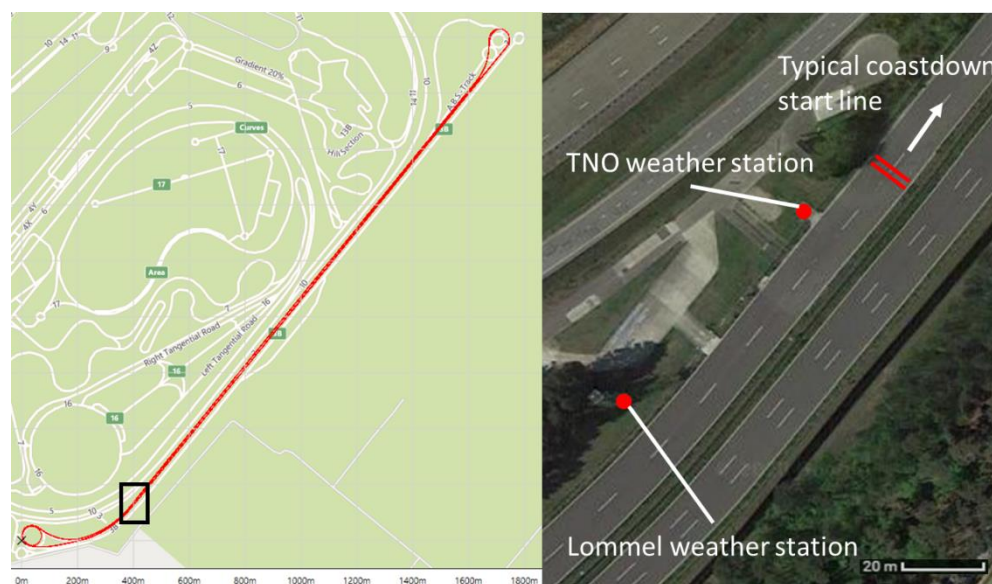
Figure 5.7: Lommel Proving Ground weather station location. The white arrow indicates the driving direction from the coast down start line (one of the driving directions).
