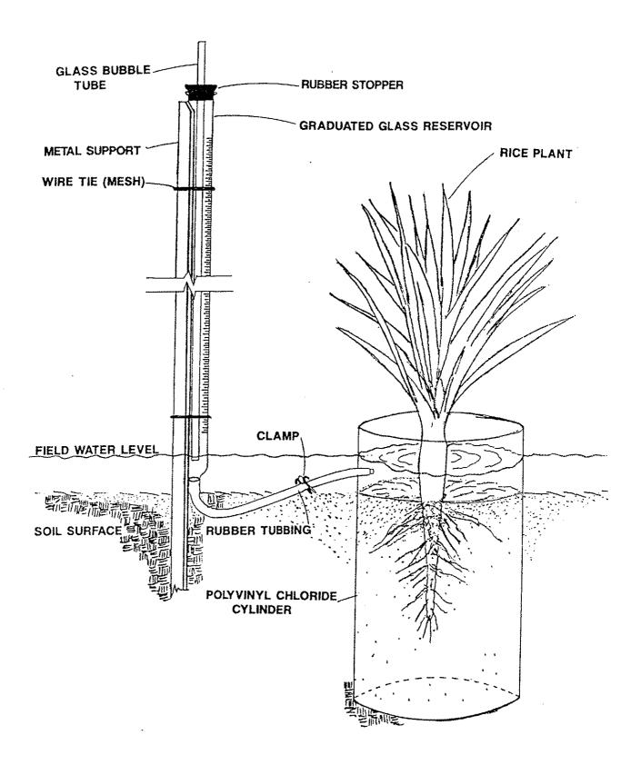
Figure 2.--A typical microlysimeter installation.
