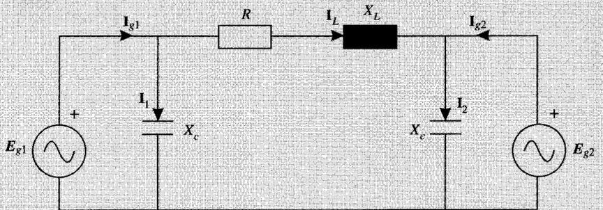
$$E_{g1} = 220/\angle 0^\circ \quad E_{g2} = 220/\angle -15^\circ \quad f = 50 \text{ Hz}$$
