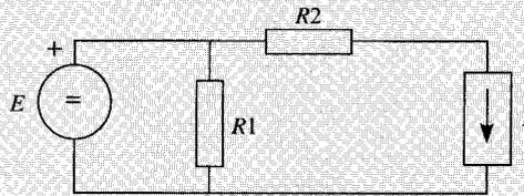
Datos:  $E = 10 \text{ V}$ ;  $R1 = 4,5 \text{ k}\Omega$ ;  $R2 = 1 \Omega$ ;  $I = 3 \text{ A}$ .
