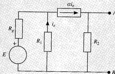
Datos:  $E = 20 \text{ V}$ ;  $\alpha = 2$ ;  $R_g = 10 \Omega$ ;  $R_1 = 5 \Omega$ ;  $R_2 = 10 \Omega$ .
