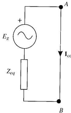
$$I_{cc, \text{máx}} \geq \frac{E_g}{Z_{eq}} = \frac{E_g}{\sqrt{\left(\frac{R_g}{N}\right)^2 + \left(\frac{X_g}{N}\right)^2}} = \frac{N \cdot E_g}{\sqrt{R_g^2 + X_g^2}}$$
