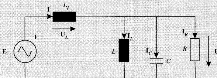
$$R = 11 \Omega; L = 45 \text{ mH}; C = 0,22 \text{ mF}; L_1 = 3,18 \text{ mH}; u(t) = 220 \sqrt{2} \cos 314,16t$$
