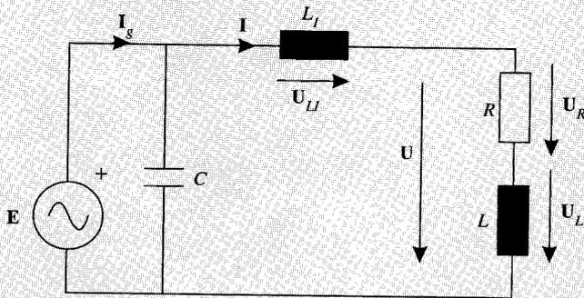
$$R = 4 \text{ }\Omega; L = 10 \text{ mH}; C = 0,64 \text{ mF}; L_1 = 1 \text{ mH}; e(t) = 230 \sqrt{2} \cos 314,16t$$
