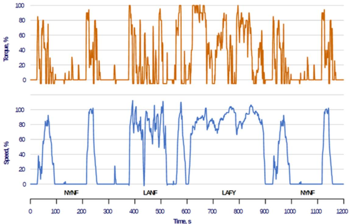
**Figure 9:** Normalized Torque and Speed of HDV FTP transient cycle (DieselNet).
