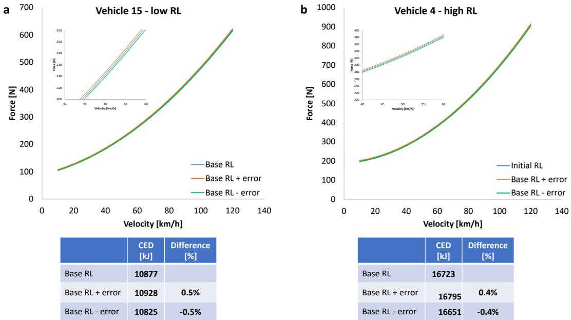
**Figure 28:** Resistance force calculation for the maximum error, (a) vehicle 15 a & (b) vehicle 4
