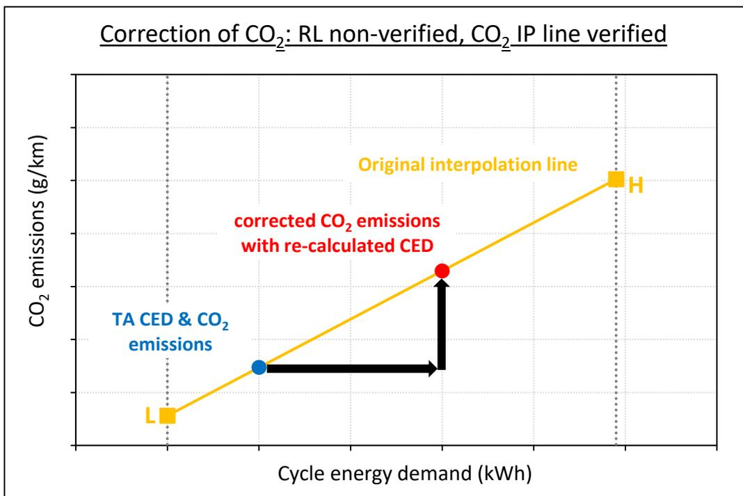
**Figure 48:** Correction of CO<sub>2</sub> emissions, in case RL is not verified and the CO<sub>2</sub> interpolation line is verified.
