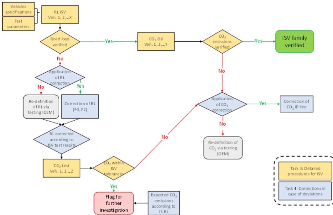
**Figure 17:** Schematic description of the sequential approach for the in-service verification procedure
