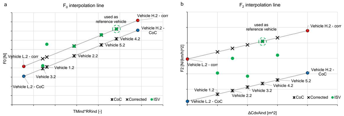
**Figure 46:** Qualitative example of the RL coefficients corrections using the vehicle with the maximum ΔCED as a reference – Option 2
