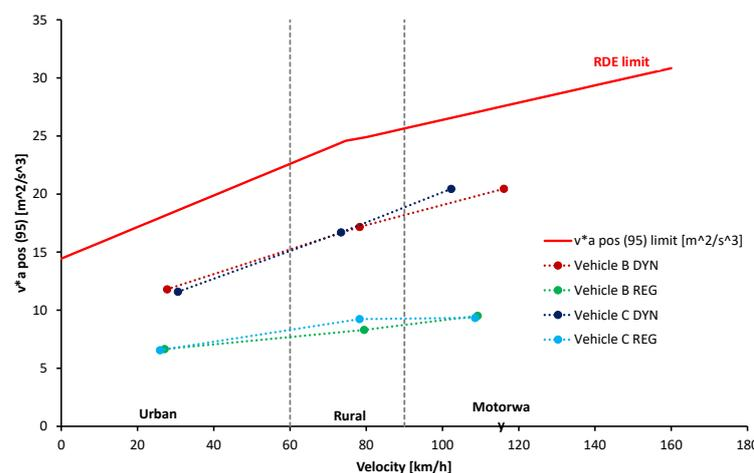
**Figure 53:** Driving dynamics for the RDE tests used in the simulation
