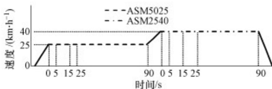
**Figure 5:** ASM2540 and ASM5025 velocity profiles.
