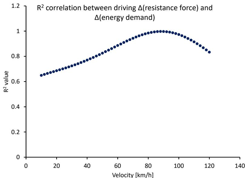
**Figure 27:**  $R^2$  correlation between driving resistance force and WLTP energy demand as function of velocity
