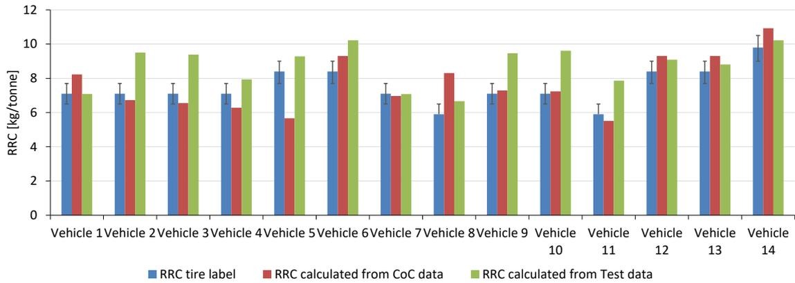
**Figure 50:** Comparison of calculated RRC and tire label
