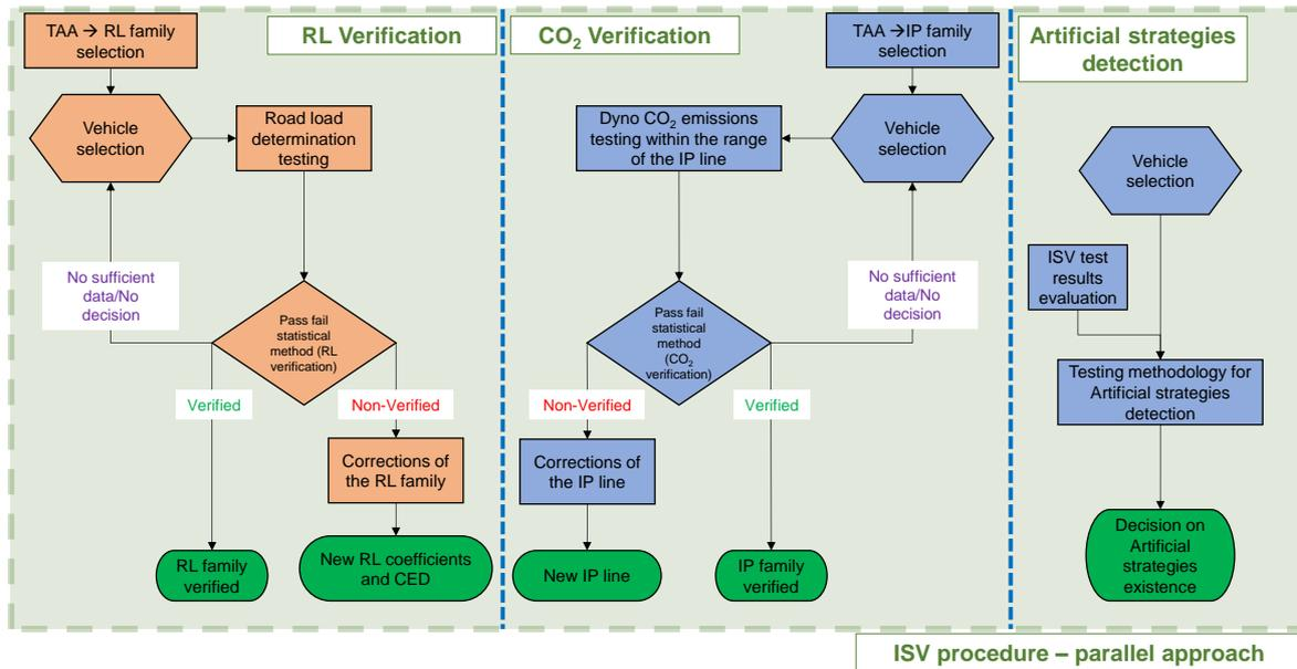
**Figure 16:** ISV procedure flowchart with RL and CO<sub>2</sub> interpolation line correction process
