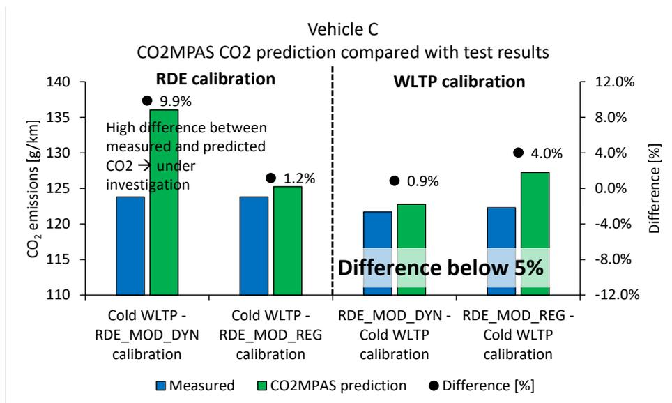
**Figure 56:** Comparison of CO<sub>2</sub>MPAS prediction and measured CO<sub>2</sub> emissions for Vehicle C
