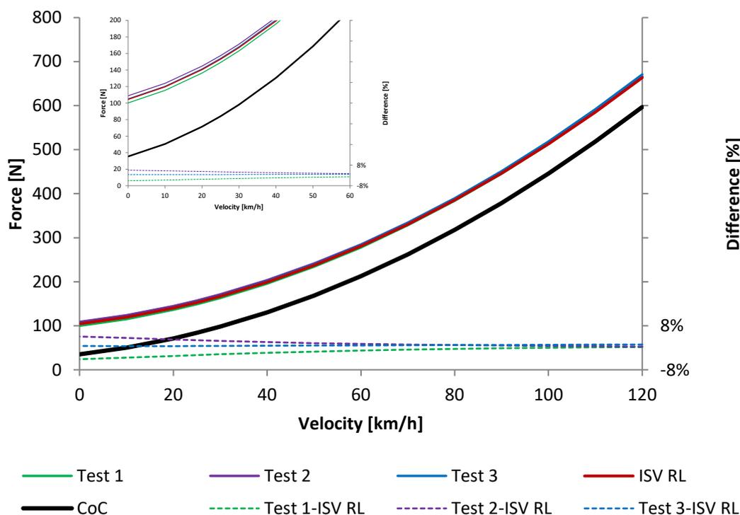
**Figure 30:** Comparison of the three repetitions of the coast down test from Vehicle 16
