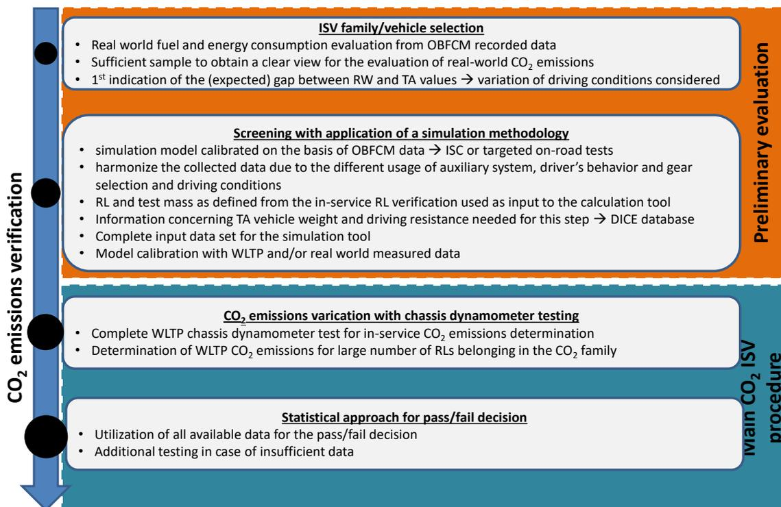
**Figure 33:** Schematic illustration of the proposed approach for the CO<sub>2</sub> verification
