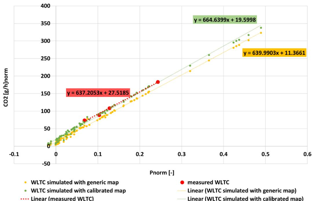
**Figure 59:** Example of measured and simulated CO<sub>2</sub> emissions in WLTC of vehicle B with calibrated CO<sub>2</sub> map, P<sub>norm</sub>: engine power normalized by P<sub>rated</sub>
