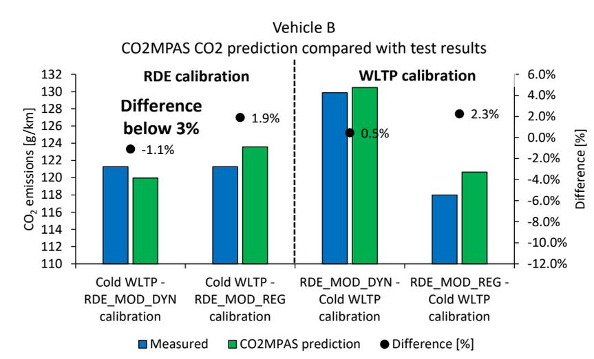
**Figure 55:** Comparison of CO<sub>2</sub>MPAS prediction and measured CO<sub>2</sub> emissions for Vehicle B
