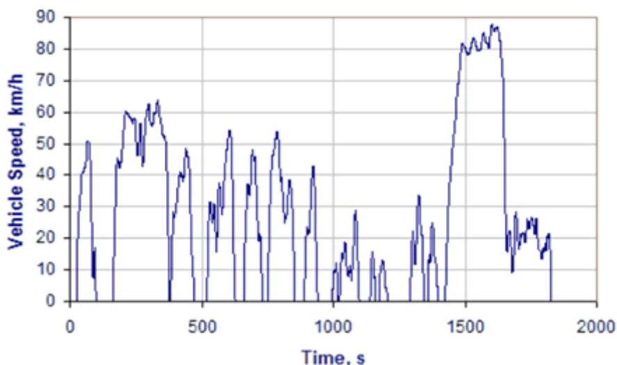
**Figure 14:** JE05 test cycle ([DieselNet](#)).
