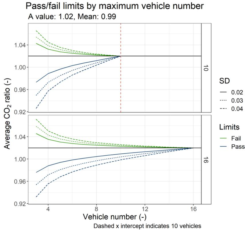
**Figure 40:** Indicative example of the CO<sub>2</sub> CoP like pass/fail statistical approach
