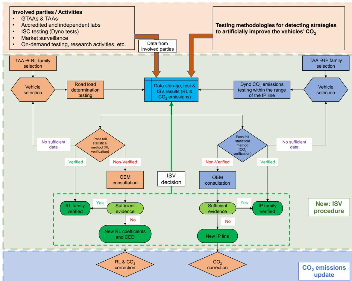
**Figure 18:** Flowchart of a possible ISV procedure
