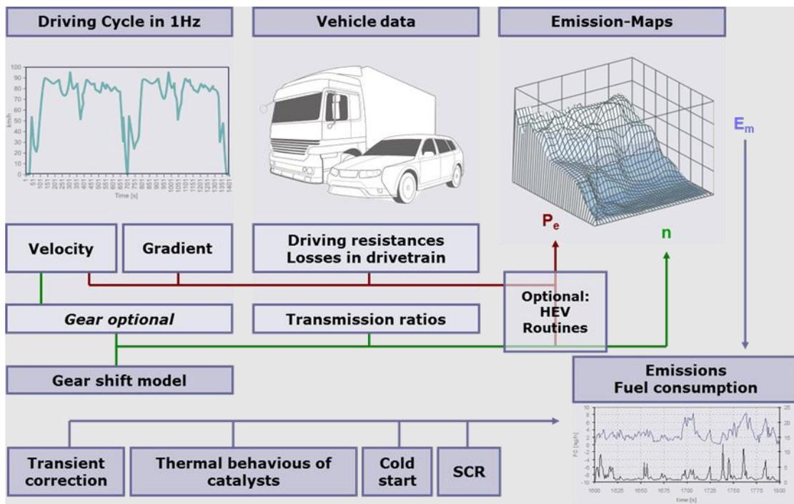
**Figure 57:** Scheme of the PHEM model
