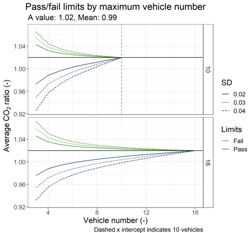
**Figure 32:** Indicative example of the CO<sub>2</sub> CoP like pass/fail statistical approach
