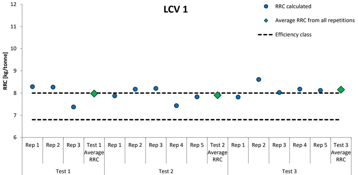
**Figure 51:** Calculation of tyre RRC and comparison with the tyre efficiency class – LCV 1
