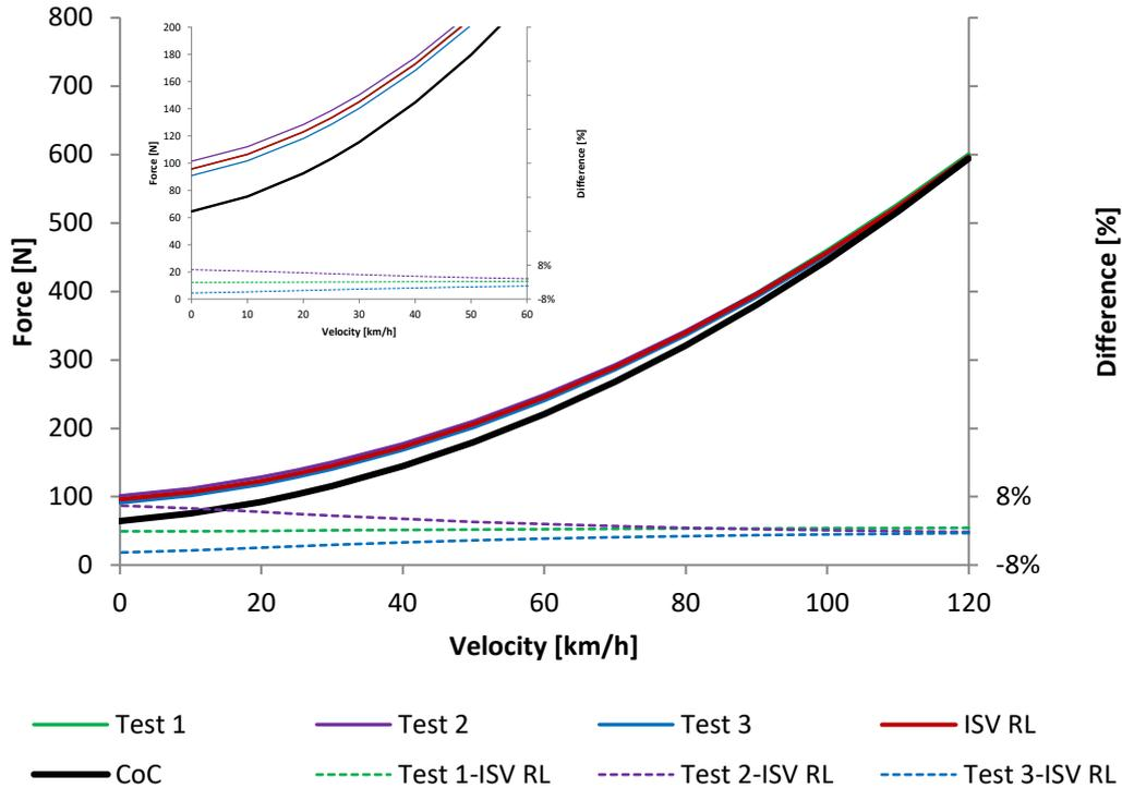
**Figure 29:** Comparison of the tree repetitions of the coast down test from Vehicle 15
