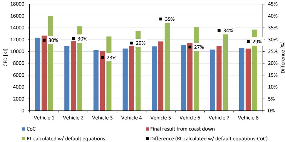
**Figure 20:** Comparison of the CED from calculated RL with equations (7) and (8), with CED from the CoC and ISV RLs
