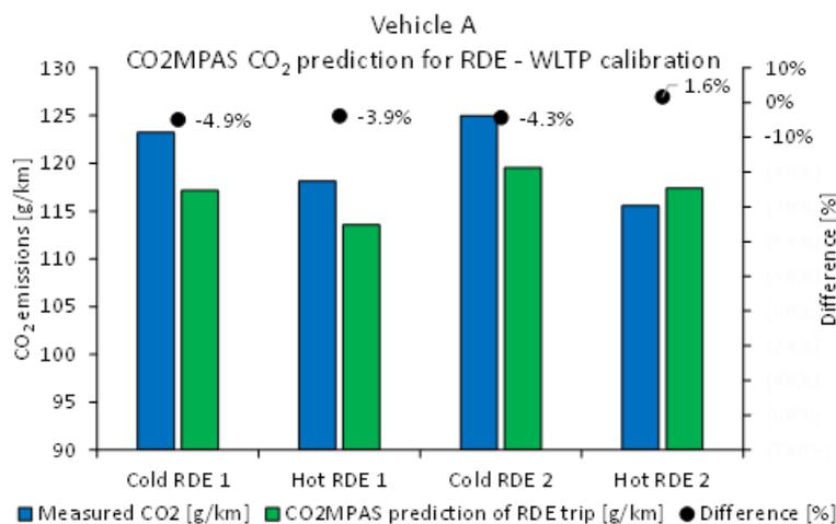
**Figure 54:** Comparison of CO<sub>2</sub>MPAS prediction and measured CO<sub>2</sub> emissions for Vehicle A
