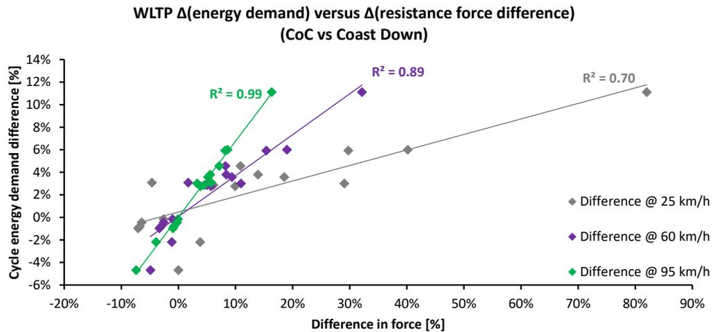
**Figure 26:** Correlation graph for driving resistance force and energy demand difference for velocity 95, 60 and 25 km/h
