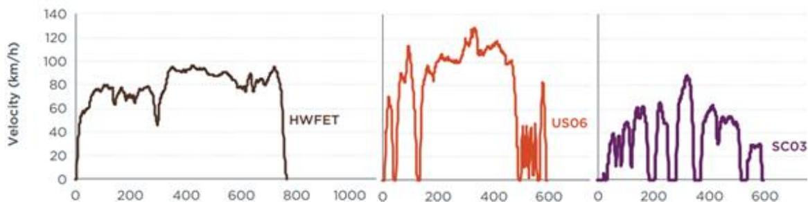
**Figure 3:** HWFET, US06, SC03 velocity profiles (ICCT 2017).
