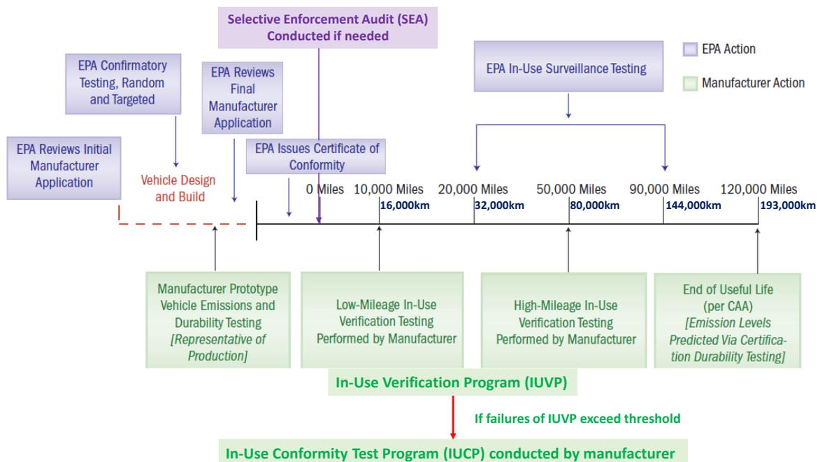
**Figure 1:** Compliance schedule for light-duty vehicles (Source: EPA 2007 Progress Report-Vehicle and Engine Compliance Activities. Oct. 2008).
