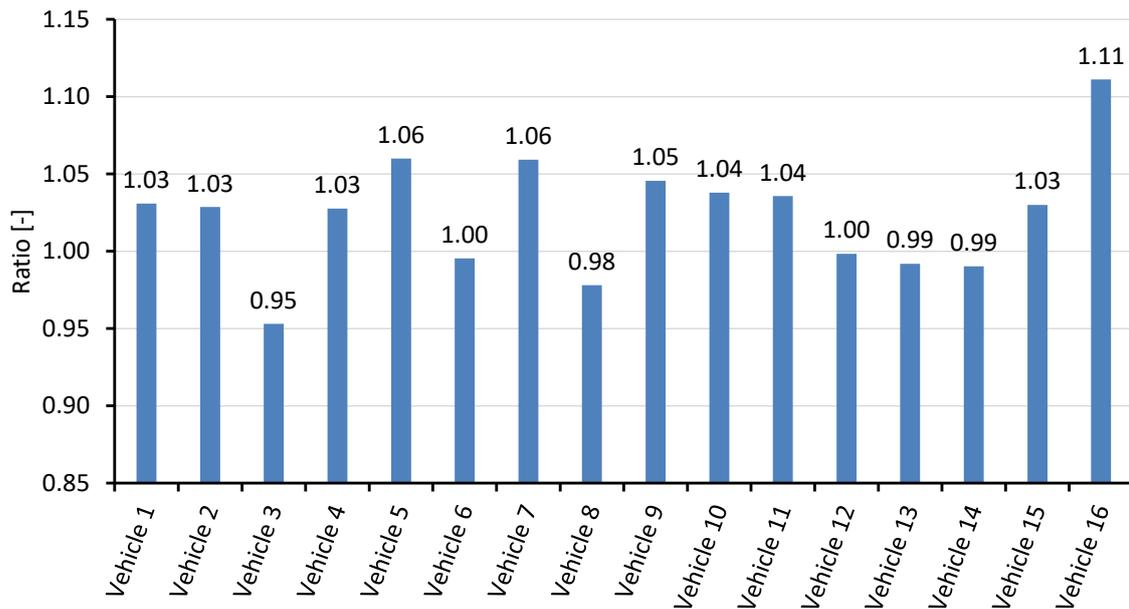
**Figure 23:** WLTP Cycle energy demand ratio of CoC & measured road loads, ratio higher than 1 (>1) indicates that the CED from measured RL is higher than the one calculated with CoC RL
