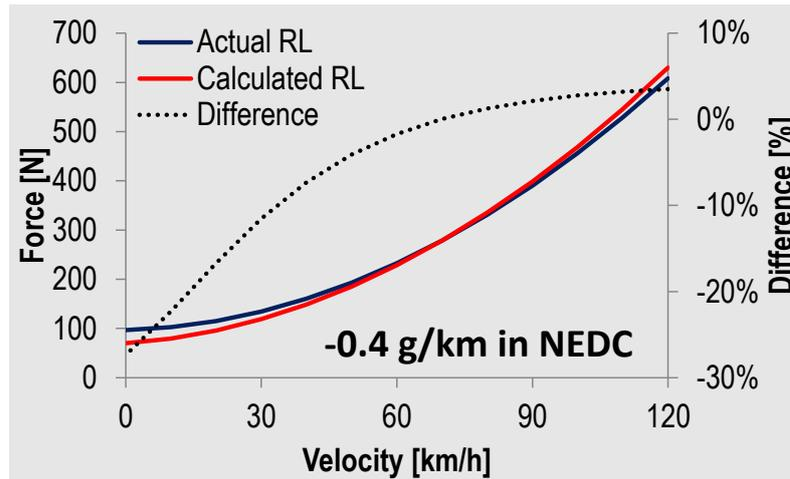
**Figure 61:** Comparison of actual and calculated RL
