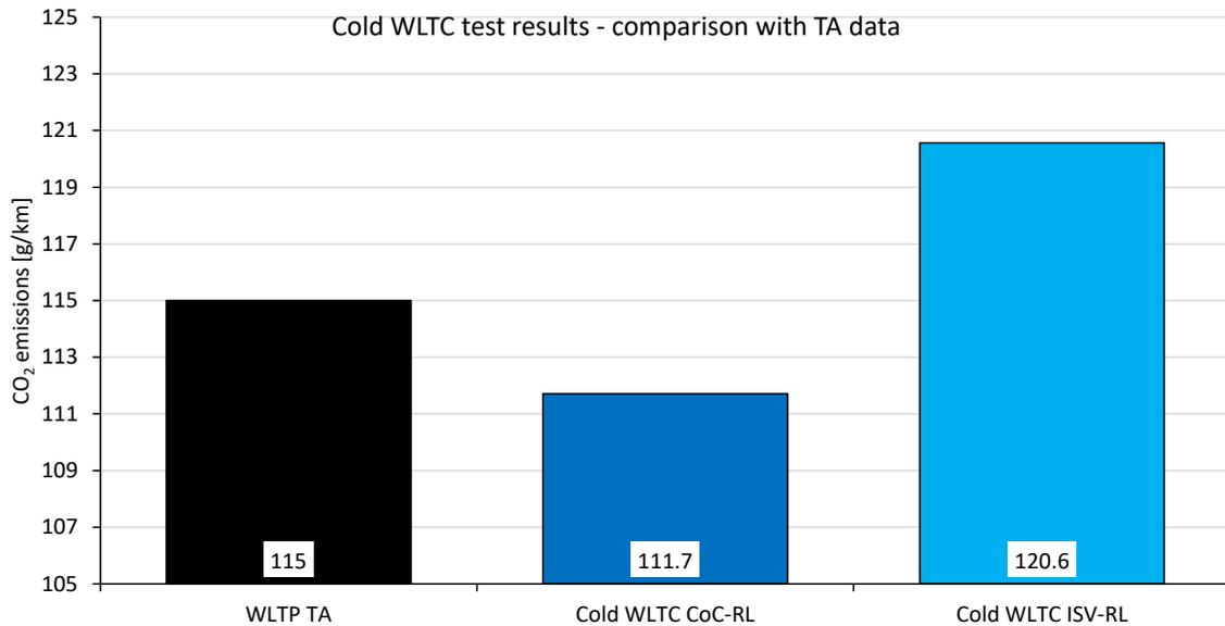
**Figure 36:** Comparison of WLTC CO<sub>2</sub> emissions results for the tests performed (vehicle 15), the total CO<sub>2</sub> emissions are calculated after the application of all corrections
