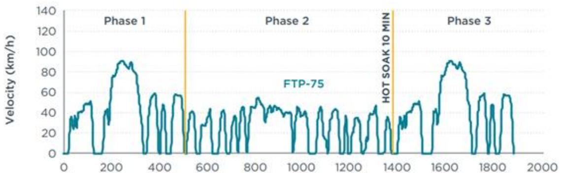
**Figure 2:** FTP velocity profile (ICCT 2017).
