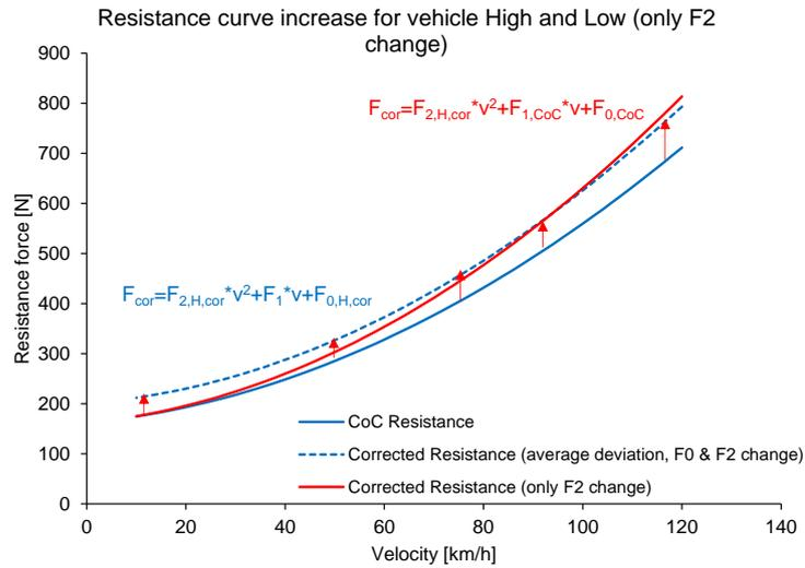
**Figure 47:** Qualitative example for the correction of the RL by modifying only the F2 coefficient – Option 3
