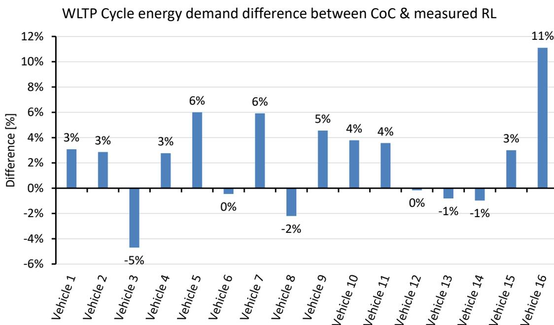
**Figure 22:** WLTP Cycle energy demand difference between CoC & measured road loads, positive difference indicates that the CED from measured RL is higher than the one calculated with CoC RL
