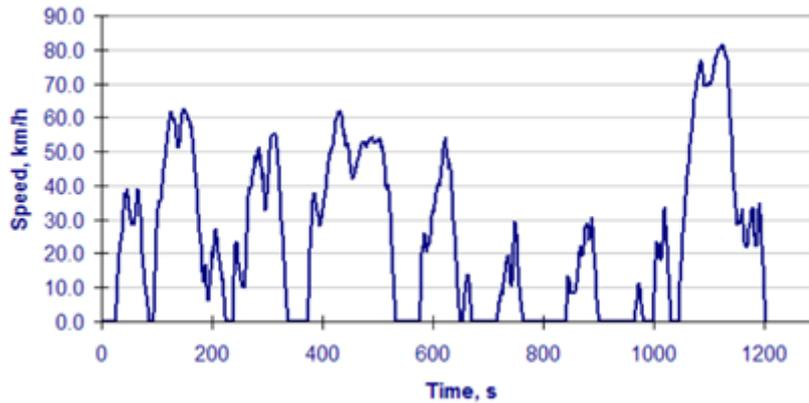
Figure 6: JC08 driving cycle ([DieselNet](#)).
