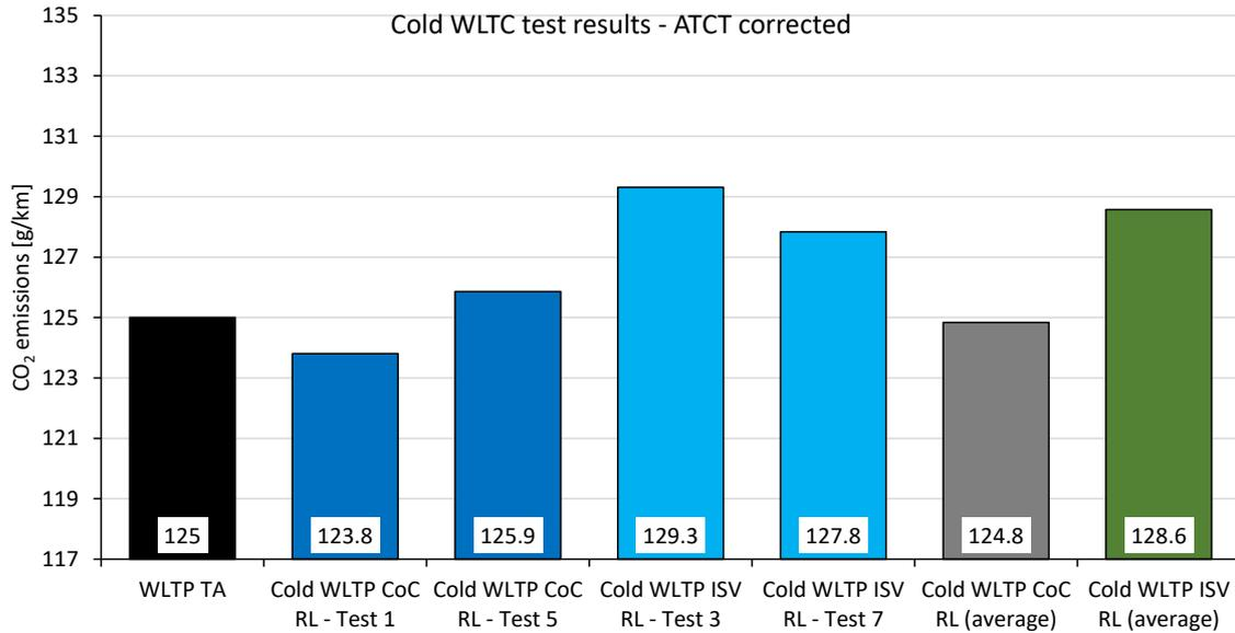
**Figure 35:** Comparison of WLTC CO<sub>2</sub> emissions results for the tests performed (vehicle 15), the total CO<sub>2</sub> emissions are multiplied by the FCF to address the ATCT correction
