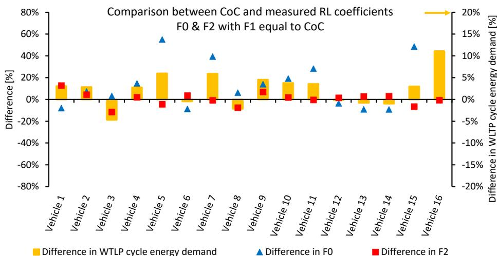
**Figure 24:** Comparison of road load coefficients for the vehicles considered in the analysis when F0 and F2 coefficients are calculated considering a constant F1, equal to the CoC (positive difference indicates that measured is higher than CoC).
