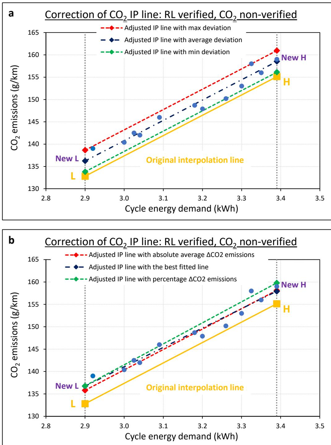
**Figure 44:** Correction of CO<sub>2</sub> IP line, in case RL is verified and deviations are found in CO<sub>2</sub> emissions (dummy data just for illustration).
