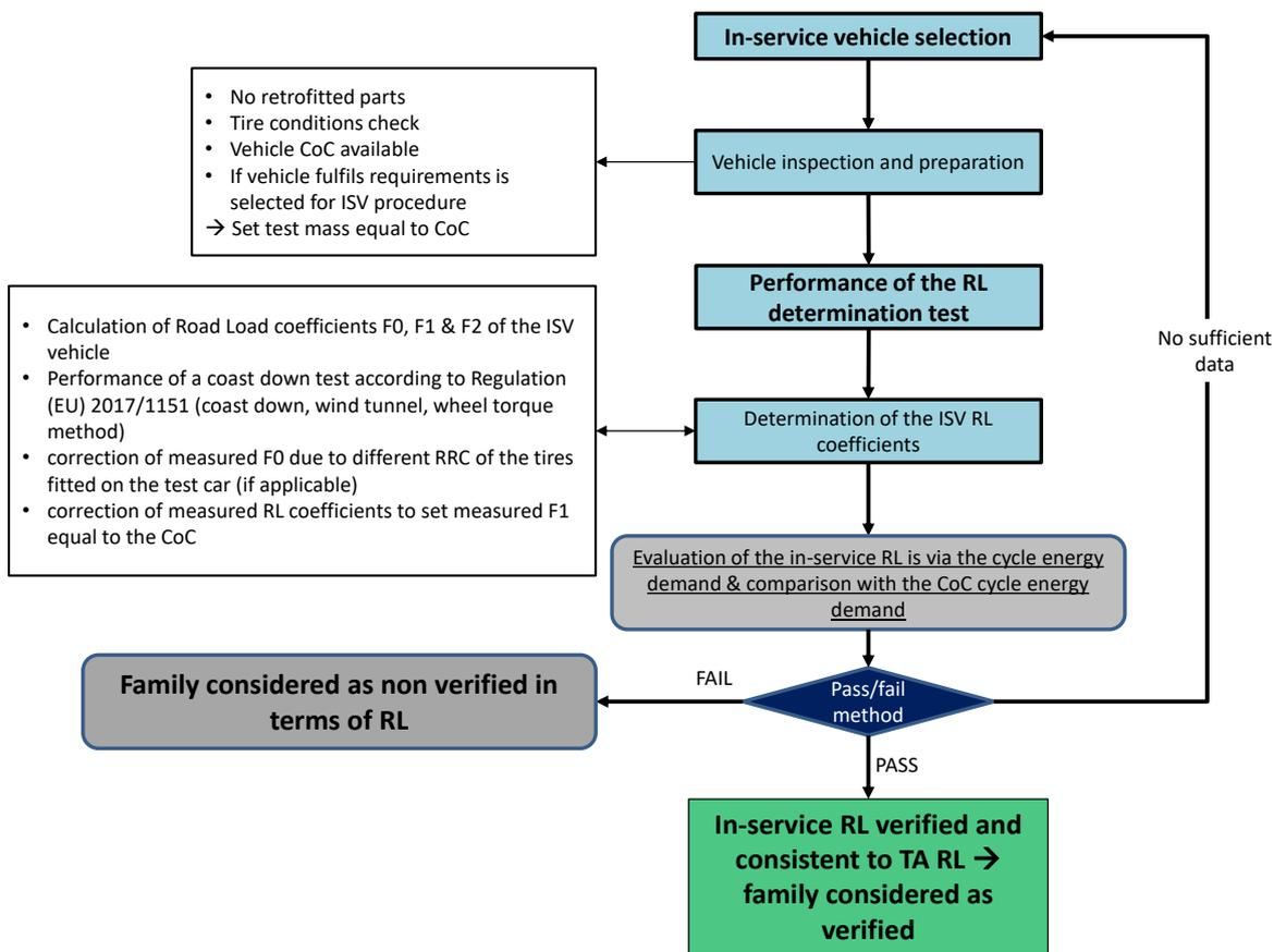
**Figure 19:** Flowchart of the proposed in-service RL verification procedure
