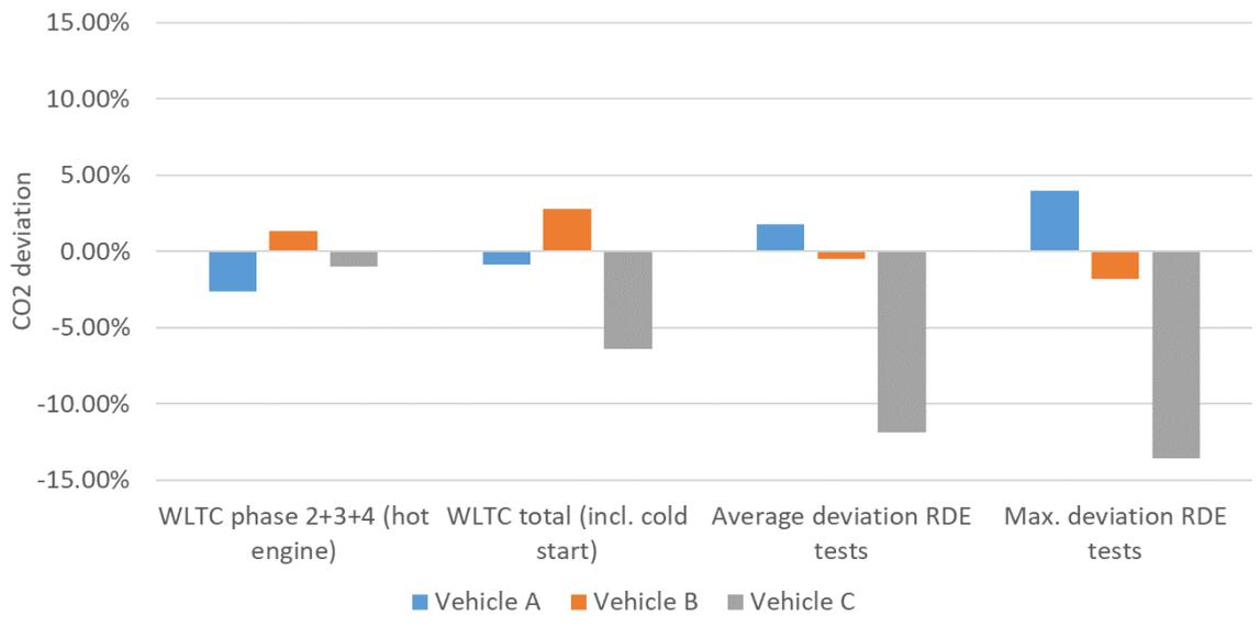
**Figure 60:** Deviations between simulated and measured cycles for vehicle A, B and C
