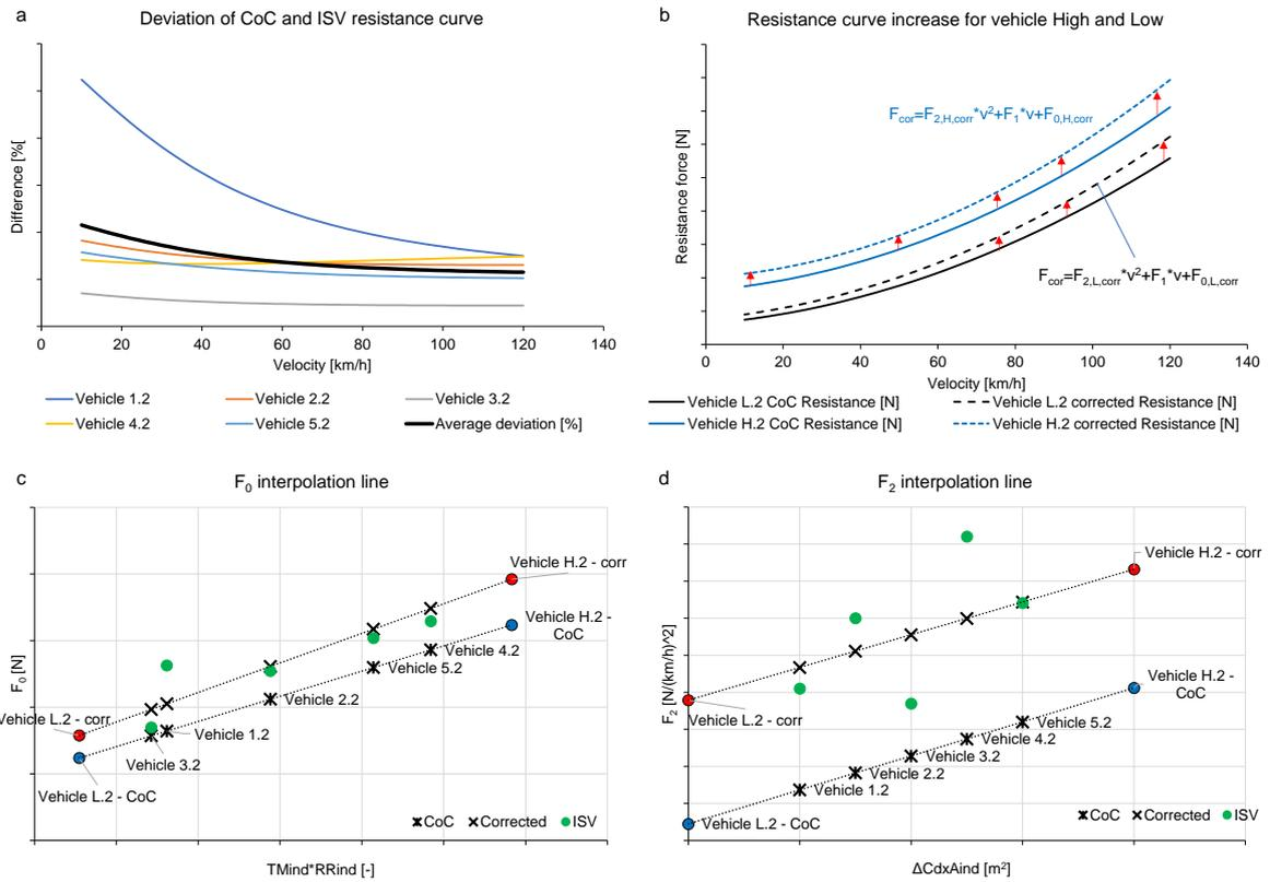
**Figure 45:** Qualitative example of the RL coefficients corrections using the average deviation – Option 1
