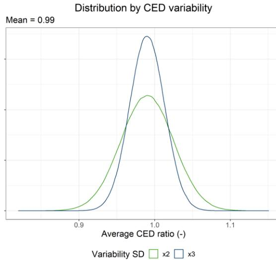
**Figure 31:** Normal distribution of CED ratio for a RL family, mean value 0.99 (indicative example), standard deviation 0.035 and 0.023.
