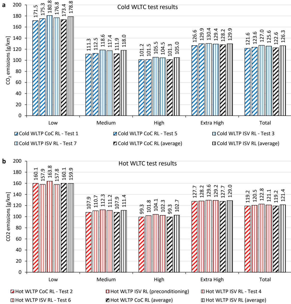
**Figure 34:** Test results for the WLTP tests of the B-segment 1.5l petrol vehicle, (a) cold start cycles and (b) hot start cycles
