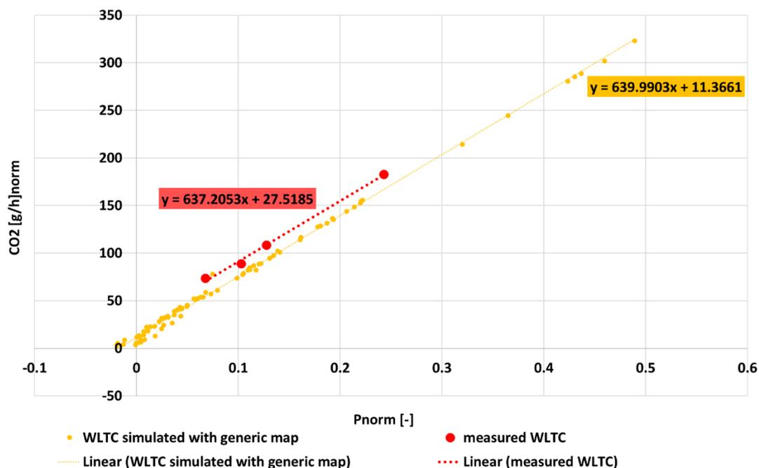
**Figure 58:** Example of measured and simulated CO<sub>2</sub> emissions in WLTC of vehicle B with generic CO<sub>2</sub> map before calibration,  $P_{norm}$ : engine power normalized by  $P_{rated}$
