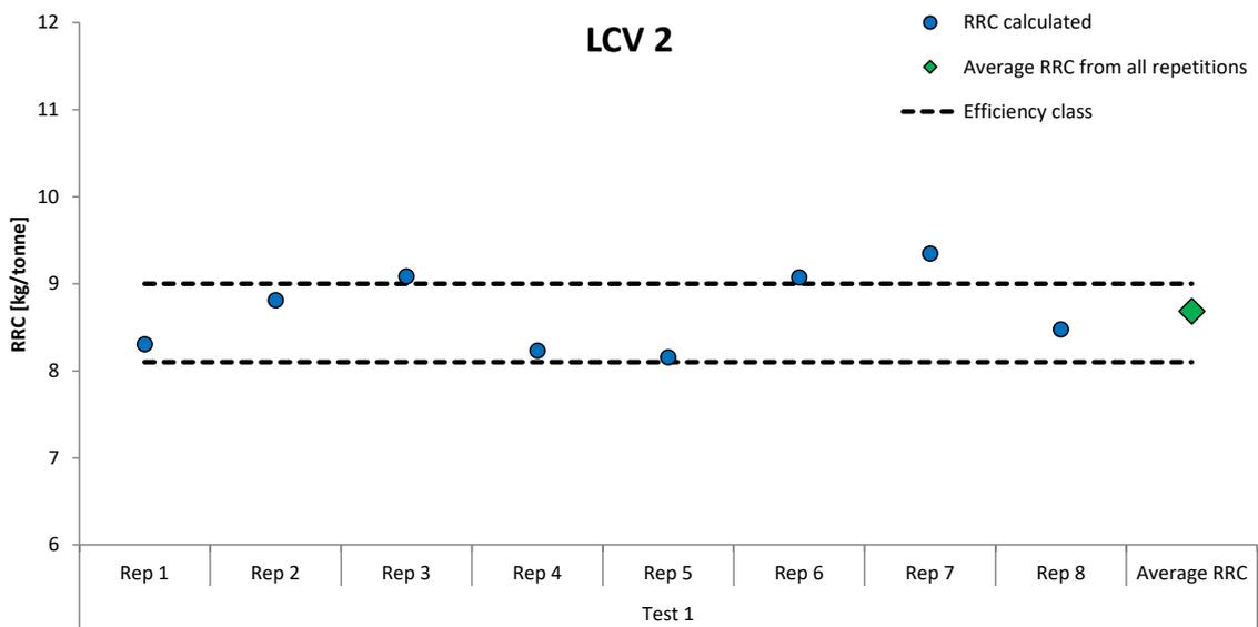
**Figure 52:** Calculation of tyre RRC and comparison with the tyre efficiency class – LCV 2
