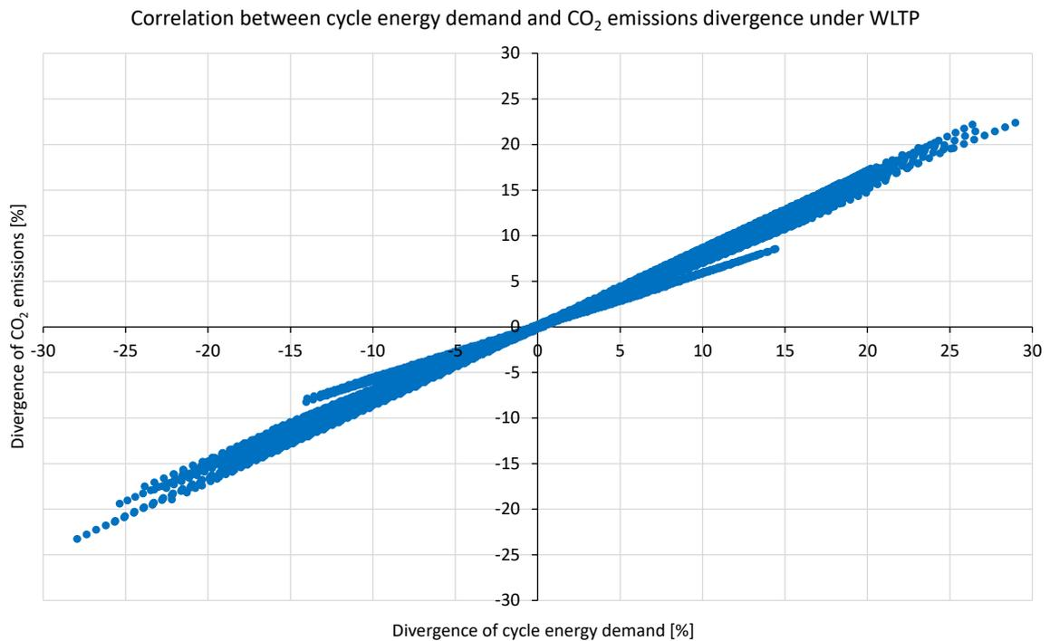
**Figure 38:** Correlation between cycle energy demand and CO<sub>2</sub> emissions divergence under WLTP for all the simulated cases
